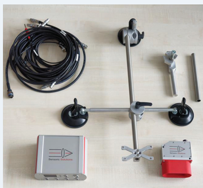
The package developed for Mercedes-Benz combines non-contact, optical technology with an IMU
